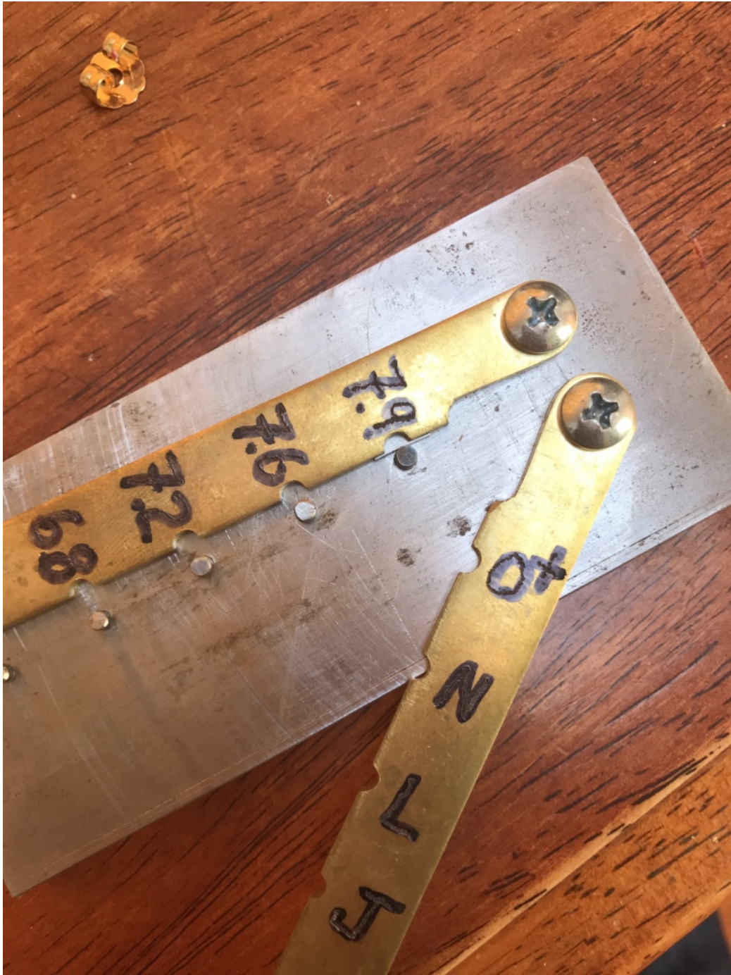
FIGURE S1. Custom-made tool for forming hummingbird bands (manufactured by Lee Rogers, Hummingbird Monitoring Network).
